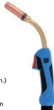
TBi 411 Classic Series 100% (10 min.) Mix: 450 A CO 2 : 500 A Ø 1.0-1.6 mm
