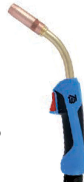
TBi 360 Classic Series 60% (10 min.) Mix: 300 A CO 2 : 330 A Ø 1.0-1.6 mm
