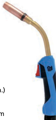
TBi 360 Classic Series 60% (10 min.) Mix: 300 A CO 2 : 330 A Ø 1.0-1.6 mm
