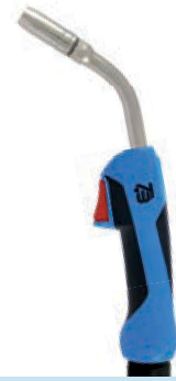
TBi 250 Classic Series 60% (10 min.) Mix: 200 A CO 2 : 230 A Ø 0.8-1.2 mm
