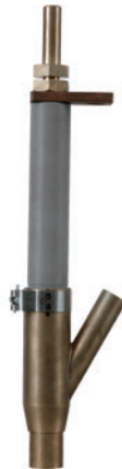
OBT 1200 043900 1,200 amps at 100 percent duty cycle. For 1/16–3/16 inch (1.6–4.8 mm) wire. Torch has concentric flux flow nozzle and features a replaceable breakaway adapter end to prevent costly damage should torch run into an obstruction.
